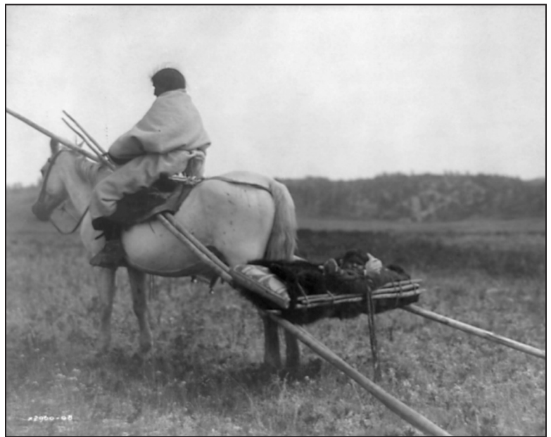
The “lodge trail” Lt. Maynadier refers to is also known as a “travois trail” for the horse drawn implement shown here. Travois served the same purpose as later-day wheeled wagons — to transport heavy loads. (Library of Congress, Edward Curtis Photograph Collection)
