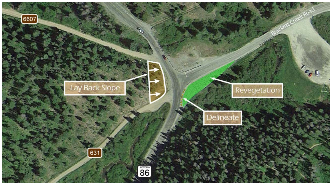
Figure 3 Brackett Creek (RP 18.8) Sight Distance Improvements
