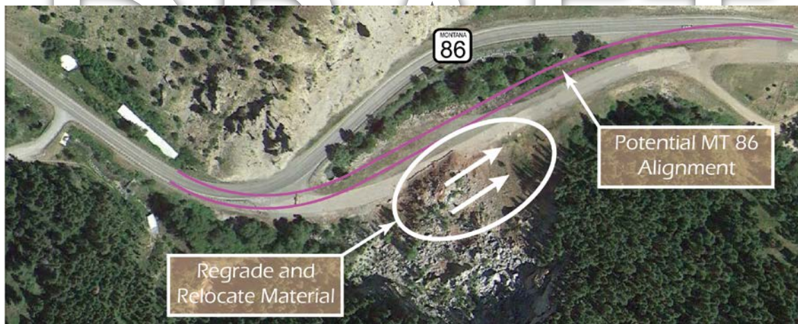
Figure 2 RP 4.3 to RP 4.6 Roadway Realignment
