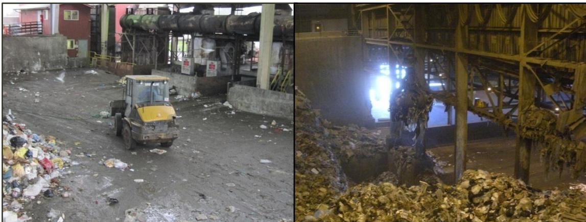
Figure 5. Combustion units loaded by a wheeled front loader (left) and overhead crane (right).
