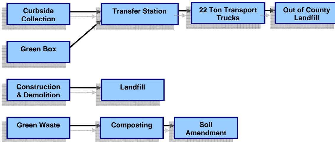
Under this scenario existing transfer station will have to be reconfigured and re-constructed to allow solid waste from collection vehicles to be deposited into the 22 ton trailers. This will require a bi-level facility whereby the collection vehicles will arrive at the upper level and drop wastes into the trailers located at a lower level.
